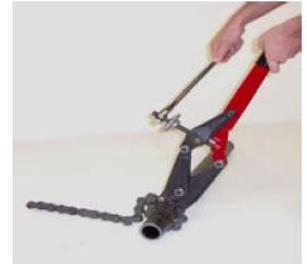
4. Place ratchet on head of drive screw and operate clockwise until pipe snaps off. If pipe has not cut before jaw wheels touch, turn counterclockwise until next pin can be engaged in jaw.
