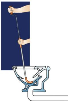
2. While turning the handle clockwise, push rod downward until the obstruction is either forced down the waste line or is caught by the boring head.
