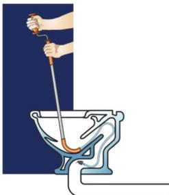
3. **IF USING TELETUBE CLOSET AUGER:** If the stoppage has not been reached, push the button located just above the grip handle, and pull back on the turning handle to release three more feet of cable, then repeat the above steps.
